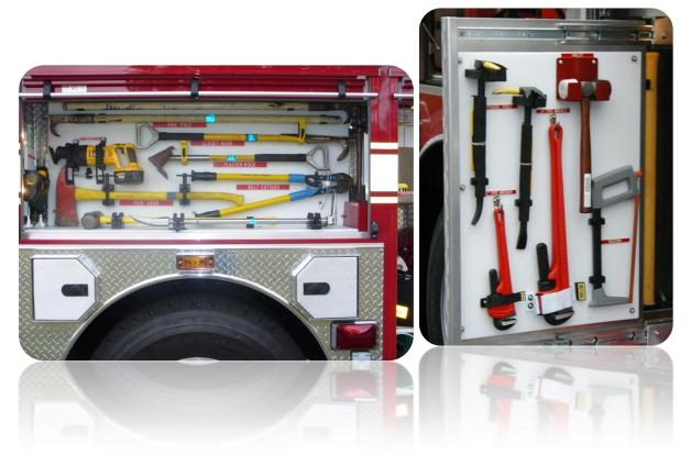
Slide out trays can be a valuable asset for heavy tools and equipment, ventilation fans, extrication tools and other equipment is able to be lifted easier from a roll out tray.
